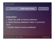
Select path to save the database, then select [Backup DB] button and press [OK] key or press [OUT] key directly to backup the database. After backup the system will prompt: "Backup DB completed!".
