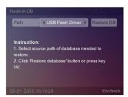
Select the database files, select [Restore DB] button and press [OK] key or press [IN] key directly to restart system.
