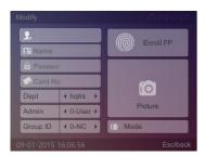
Enter the ID and press [OK] key to confirm, the user information display automatically then could modify the user information. After finished, press [Esc] key to save the modification for user.
