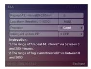
[Repeat Att. interval (0-250m)]: The same user time interval between the two time attendance, default 0 (no interval). The setting range is 0-250 minutes.
