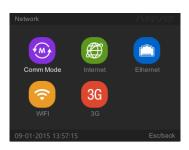
Include types of communication settings of the communications, real-time monitoring, access to IP, the network interface type setting and parameters of the machine's network settings. Settings steps as: [Comm mode]  $\rightarrow$  [Internet]  $\rightarrow$  [Ethernet] or [WIFI].
