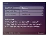
[FP verify first]: The response of the device when user first use registered fingerprint comparison on the device. There are four modes:
