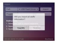
Press [OK] key to confirm import the user information. Press [Esc] key to exit. After import is completed, the system prompts 'Import successfully'.
