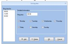
Set the desired time bell rang the bell at the time of the entry box. Click [+ Add] button to add time to time list. When the time list for invalid bell time, you can delete the invalid time. Select left invalid ring time, click [-Delete] button to bring up the dialog box to confirm the deletion:
