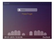
Put the fingerprint on the FP sensor to register. (Scan the same finger twice to enroll the fingerprint. After registering first, the system will prompt 'Press Finger Again':
