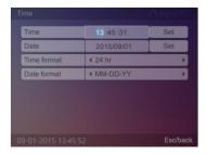
Adjust the time and date, select [Set] button and press the [OK] button to confirm the settings take effect.
