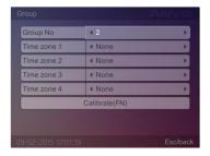
Select the group number, then the time zone of the group corresponding, such as the group 2 include the timezone is 1, after completion click [Calibrate(Fn)] or [F1] key to make the settings take effect.
