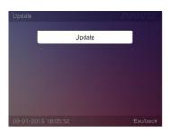
Insert USB flash driver which has firmware file, then press [OK] key to update, we can press [Esc] key to return a higher level interface.
